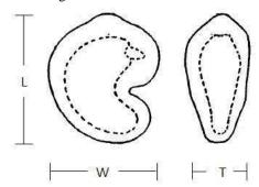
Figure 1: Length(L) ,Width(W) and Thickness (T) of the cashew kernel.
